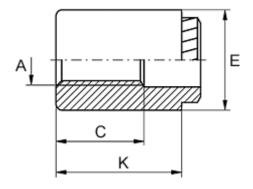
Female thread A = M2 Height K = 11 Hole diameter +0.1 = 3.7 Min distance to edge = 2.2 Min material thickness = 1.5 Outer diameter E = 6 Thread length = 9
